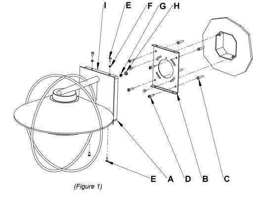
**IMPORTANT:** Wall mount bracket must be secured to a solidly mounted electrical box and/or a framing member in at least two locations. Do not depend on drywall anchors alone to support this fixture. If in doubt, contact a qualified electrician.
