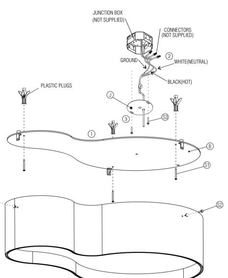
Turn off the electrical power before starting the installation, and keep it turned off until the installation is completed.
