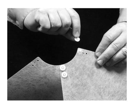
**Step 6** Fold the shade panel (O) as shown to match the "C" sides. Insert the other side of the shade panel (O) onto the two male end plastic buttons (P).
