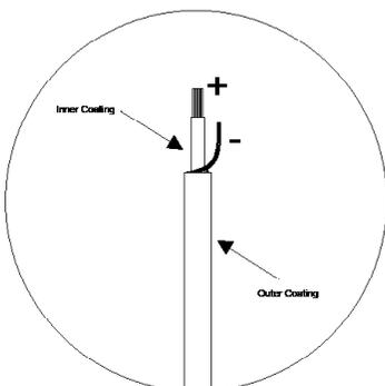
Coax cable requires stripping of outer and inner coatings to access positive and negative connection wires
