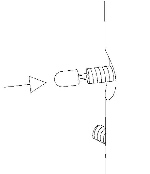
2. Twist glass orbs onto threaded rods
