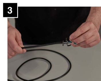
Feed lock washer and nut/balancer through cord.
