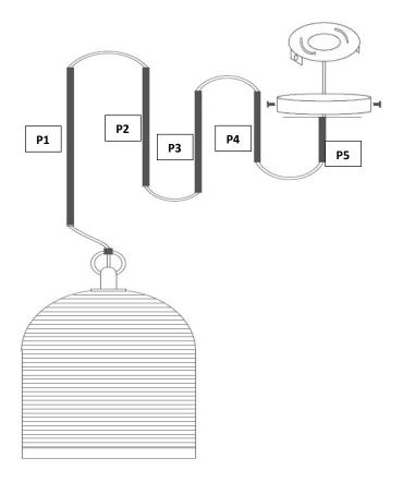
• Gently pull the slack cable out of the canopy until the assembled poles meet the thread of the Shade Fixture (H). Screw the lower pole into the shade fixture. Ensure that the poles are turned clockwise until it is secured. Hold the shade fixture stationary and rotate the pole to prevent twisting of the cable.
