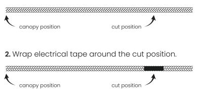
**3.** Cut the cord in the middle of the electrical tape. and continue to assemble and install the fixture as shown in the instructions.
