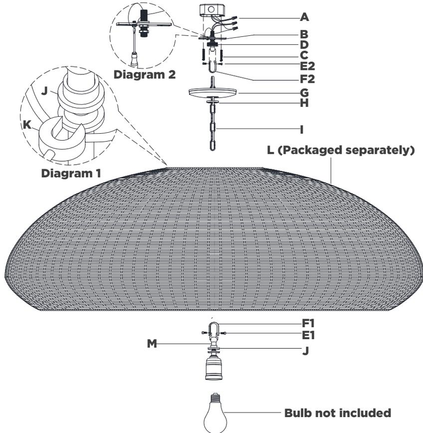
19. Install canopy **(G)** to collar loop **(D)** and secure with collar ring **(H)**.
