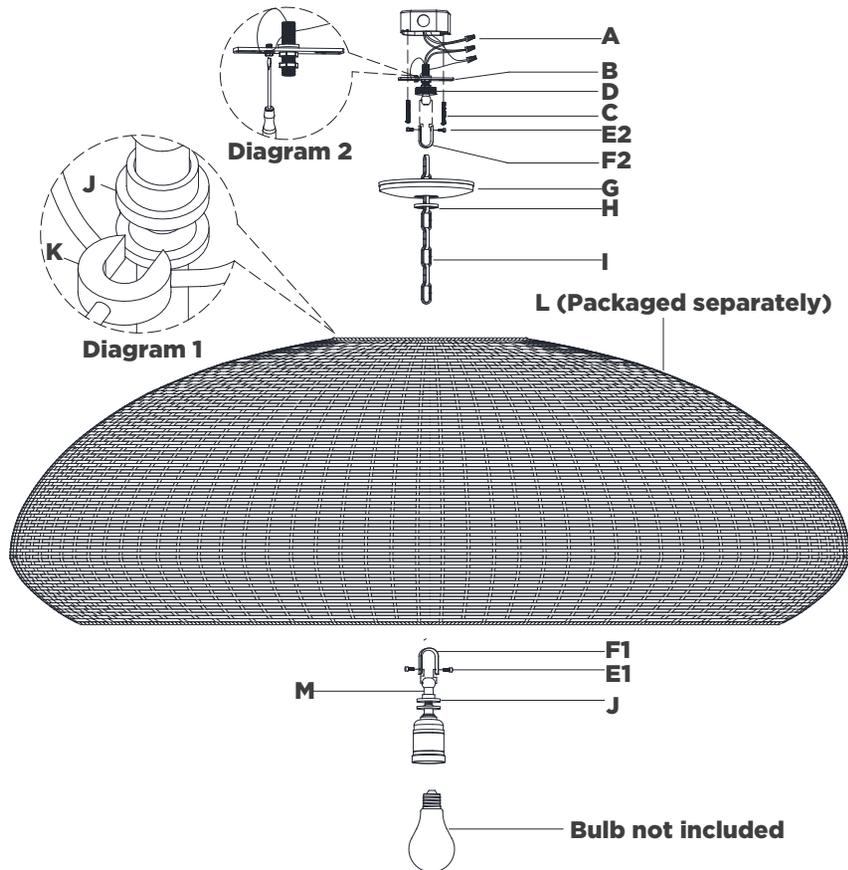
11. Thread fixture wire and ground wire through chain **(I)**.
