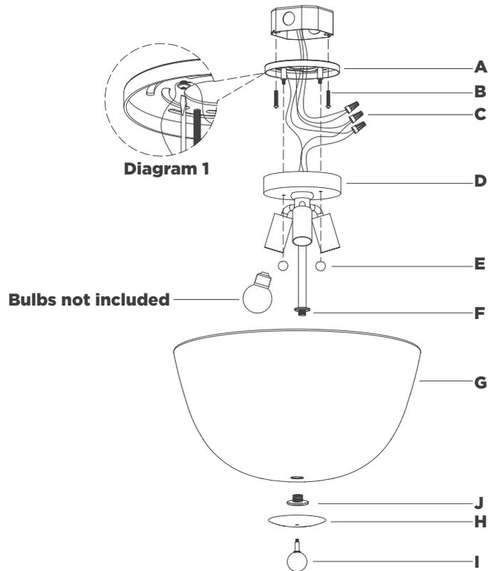
9. Install light bulb into the socket.
