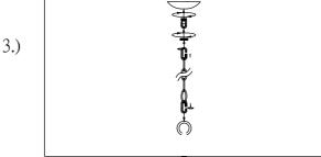
Step.3: Remove ring from top and slide down chain. Place canopy (D) onto chain (C) and let slide to top of fixture. Install nipple and cross bar into top of chain loop.
