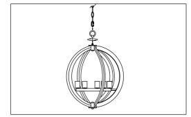
Step.2: Install top loop (A) to body (B) and attach appropriate amount of chain to loop to achieve desired mounting height. Thread wire through every 3rd loop of chain.
