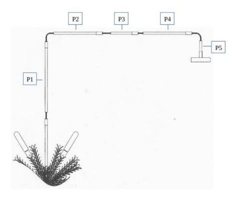
• Gently pull the slack cable out of the canopy until the assembled poles meet the thread of the Pendant Top Pole (H). Screw the lower pole into the Pendant Top Pole. Ensure that the poles are turned clockwise until it is secured. Hold the Pendant Top Pole stationary and rotate the pole to prevent twisting of the cable.
