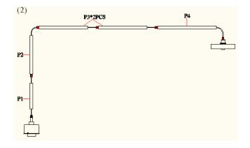
Gently pull the slack cable out of the canopy until the assembled poles meet the thread of the Socket Fixture (H). Screw
