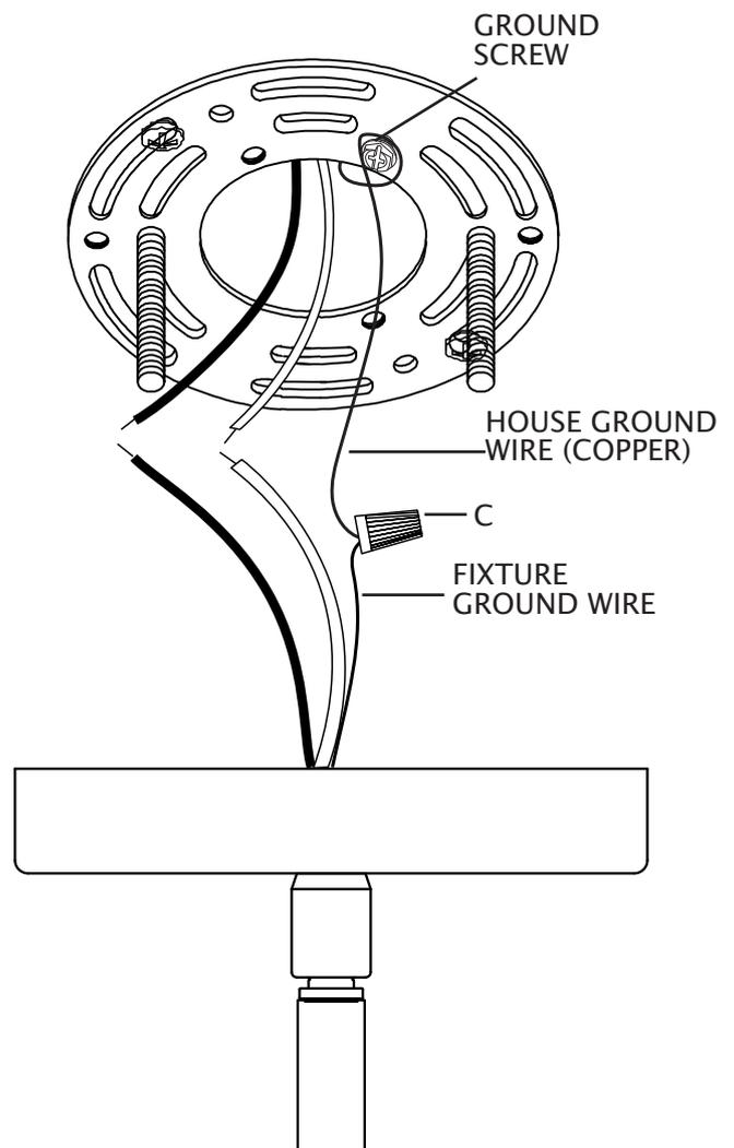
15. Twist end of house lead wire (black) and end of fixture lead wire together. Twist wire nut (C) onto ends of wires. Completely tighten wire nut (C). Twist end of house neutral wire (white) and end of fixture neutral wire together. Twist wire nut (C) onto ends of wires. Completely tighten wire nut (C). Reference chart to the right for correct wire connections.
