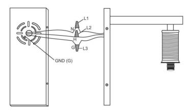
c) Connect the GROUND WIRE of the fixture to the GROUND J-BOX WIRE (usually green or bare). Fasten each together with a wire connector (L) and wrap the connection with electrical tape. Be sure that no wire strands are exposed. If there is no ground wire in the J-Box, use a screwdriver to secure the end of the fixture ground wire to the Ground screw (G) into the back plate (C).
