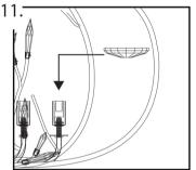
Slide one bobesche onto each socket in the fixture
