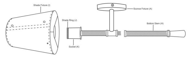
Hold the Sconce fixture stationary, screw the Bottom Stem into the Sconce Fixture and rotate the Bottom Stem clockwise until secure.
