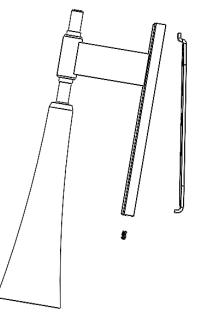
**Step 6**: Attach glass by screwing glass retention and blown glass assembly onto the LED mount inside of the cover.
