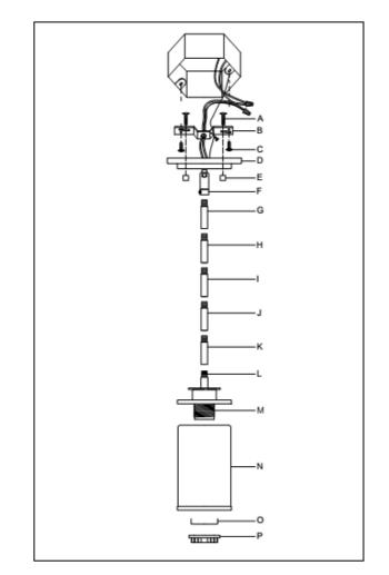
Line art shown may not exactly match the fixture enclosed. However, the installations do apply to this fixture. ITEM NO:412MP 413MP
