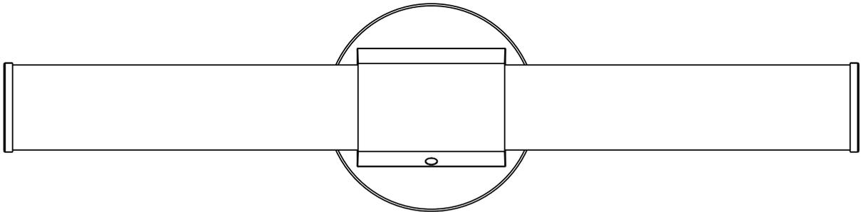
Lamping | Ampoule: 1 x AC LED 20W ( Included )
