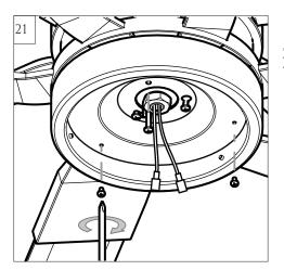
Removed set screws from light pan. Keep screws.
