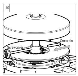
Helpful hint: For easy assembling of the cross pin on the next installation step. After slip downrod into the motor yoke, carefully insert a Phillips screwdriver through the yoke and downrod (don't damage the lead wires) as a guide and then push the cross pin and pull the screwdriver in the meantime as shown in the inset.
