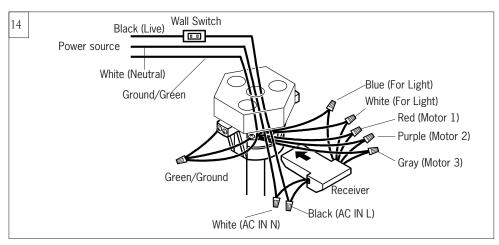
Make wiring connections using wire connectors provided as indicated above. Red from fan to Red from remote marked Motor 1. Purple from fan to Purple from remote marked Motor 2. Gray from fan to Gray from remote marked Motor 3. Blue from fan to Blue from remote marked FOR LIGHT. White from fan to White from remote marked FOR LIGHT. White (Neutral) from house to White from remote marked AC IN N. Black (Live) from house to Black from remote marked AC IN L.
