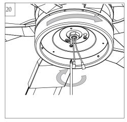
Install the light pan. Align its key holes with the set screws on the plate and reinstall the screw removed in step 18. Tighten screws securely.
