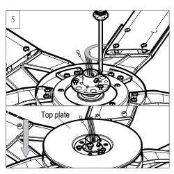
Partially loosen the 3 set screws on the yoke as shown in the illustration. Install a top plate. Place top plate over lead wires and safety cable. Align the 3 key holes on the plate with the preinstalled screws on yoke and turn clockwise till tight. Tighten screws securely.
