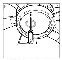
Attach LED light fixture onto the light pan, aligning the holes on the LED light fixture with the screw holes on light pan. Reinstall the screws removed in step 21. Tighten all screws securely.
