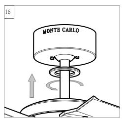
Lift canopy up, aligning its keyhole slot with the preassembled screw on mounting bracket and twist counterclockwise to lock in place. Reinstall the screw removed in step 15 and tighten all screws securely. Attach canopy bottom cap onto canopy by aligning its notch with the screws on mounting bracket and twist clockwise till tight.
