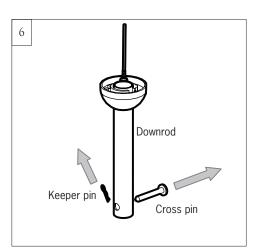
Remove preassembled keeper pin and cross pin from downrod. Keep parts.
