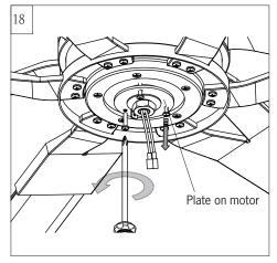
Loosen 2 and remove one set screws from the plate on motor as shown in illustration. Keep screw.
