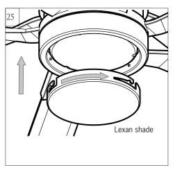
Attach lexan shade by locating dimples in light pan with grooves on the Lexan shade and twist clockwise until tight.
