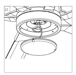
**Caution**: Corresponding to next installation step, tuck the lead wires into the light pan as shown in illustration and make sure the light lead wires are not pinched between the light pan and the LED light fixture.
