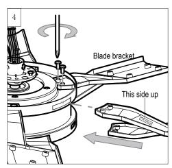
Place motor assembly on a suitable area of Styrofoam and Install blade brackets. Insert blade bracket into the slots on flywheel, aligning the holes on blade bracket with the screw holes on flywheel (**both top and bottom sides**), and then partially install set screws provided.
