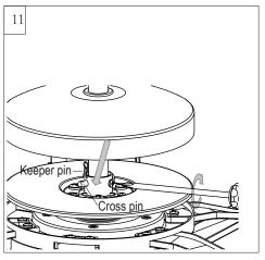
Slip downrod into motor housing yoke, aligning holes and install cross pin and keeper pin.
