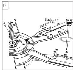
Install blades. Align the holes on a blade with screw holes on blade bracket and install it with screws provided. Tighten screws securely. Repeat this process with remaining blades.
