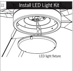
Connect white wire from fan to white wire from LED light fixture and then connect blue (or black) wire from fan to blue (or black) wire from LED light fixture.
