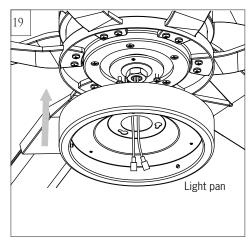
Place light pan over lead wires
