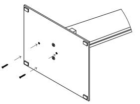
**6.** Following the installation of the fasteners in step 6, insert the two wood screws and tighten them.
