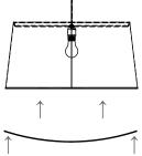
**NOTE:** For uninstallation of lower diffuser gently lift up one edge of the lower diffuser and carefully bend the diffuser until it can be removed from the bottom of the shade assembly.
