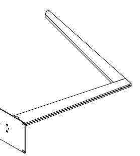
**5.** Once the base is in position, insert the two 1/2-13 flat head socket screws and tighten using a 5/16" hex key.
