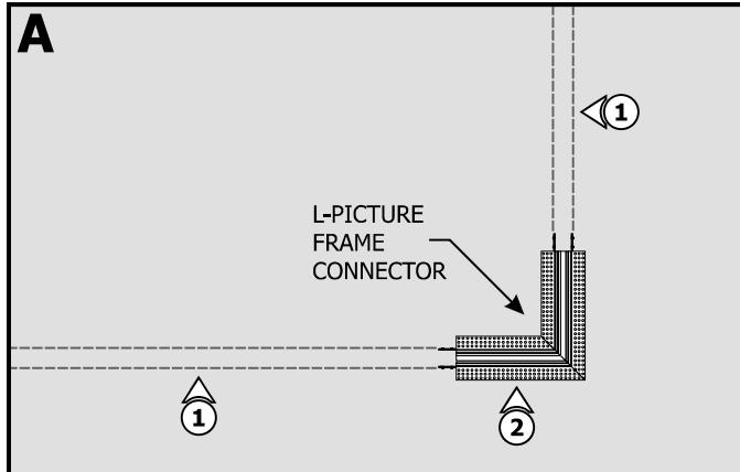
**1:** Place the L-Picture Frame Connector against the wall. Ensure the L-Picture Frame Connector is aligned with the TruCurve or TruArch Channel installation location.
