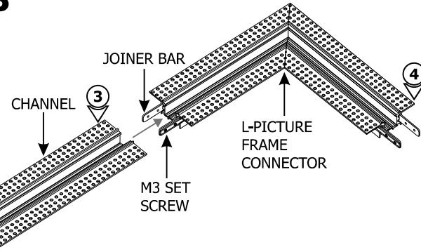
**3:** Slide a channel into the joiner bars and tighten the remaining M3 set screws using a 1.5mm Allen wrench.
