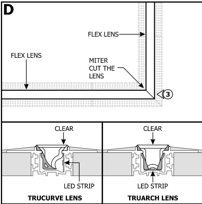
**1:** Determine the length of the lenses. Allow the total length to be 1/2" longer to avoid light leaks.
