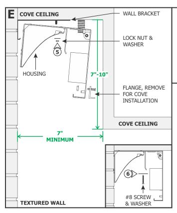
**NOTE:** For a cove (7" - 10") installation, remove the flange for a tighter fit installation.
