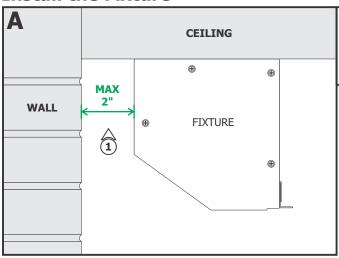
1: Depending on the design of the wall texture, it is recommended to power a section of the Stratus, hold it against the ceiling and next to the wall. Move the fixture maximum 2" away from wall to find the best grazing option for the textured wall.
