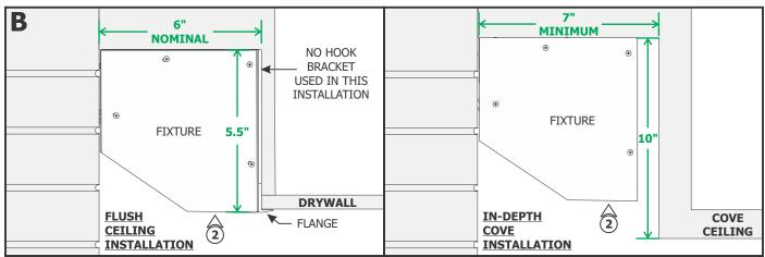
2: Determine the location where the fixture will be installed. In most cases, the fixture will be installed in either a flush ceiling or in a in-depth cove installation.
