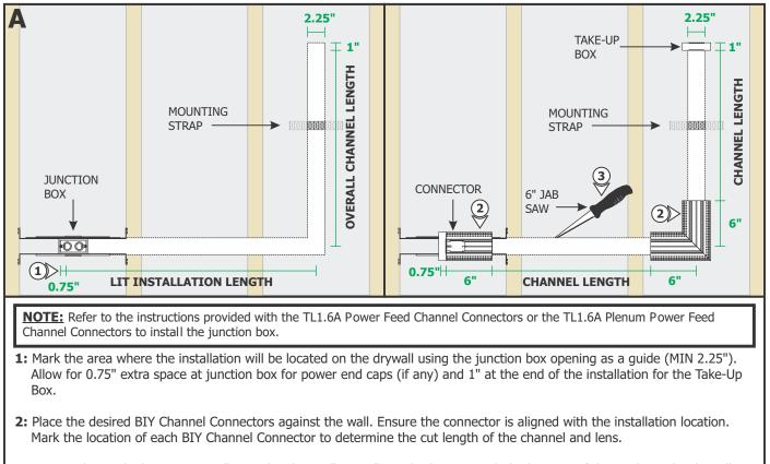
3: Cut out the marked area using a "Dremel Multi-Max" or a 6" Fixed Jab Saw. Mark the location of the studs on the drywall.
