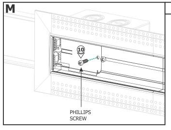
**10:** Replace the trap door and secure using the Phillips screw.
