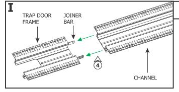
**4:** Slide a channel onto the joiner bars and tighten the two M3 set screws using a 1.5mm Allen wrench.
