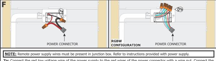
**7a:** Connect the red low voltage wire of the power supply to the red wires of the power connector with a wire nut. Connect the black low voltage wire of the power supply to the black wires of the power connect with a wire nut.
