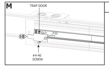
**10:** Replace the trap door and secure using the #4-40 screw with a 1/16" Allen wrench.
