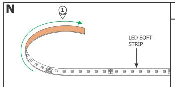
**1:** Gently uncoil the LED Soft Strip before applying to the channel otherwise the strip may lift off of the surface.
