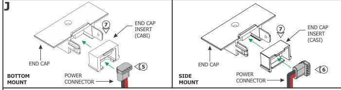
**5:** For installations where the LED Soft Strip will be laid on the bottom of the channel, place the power connector into the end cap insert (CABI).
