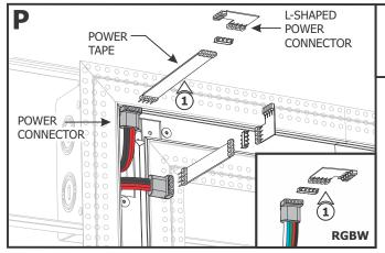
1: Refer to steps 1 through 4 in Section Three to uncoil the LED Soft Strip and connect each power connector to the Blank Power Tape (not used with RGBW), Power Adapter and L-Shaped Flexible Connector.
