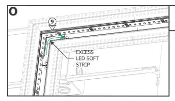
**9:** Trim excess LED Soft Strip ONLY at dashed cutting lines. Overlap excess LED Soft Strip at power connection to avoid dark spots in installation.
