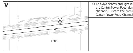
**1:** To avoid seams and light leaks, use the whole lens to cover the Center Power Feed along with the rest of the installed channels. Discard the precut lens that was provided with the Center Power Feed Channel.
