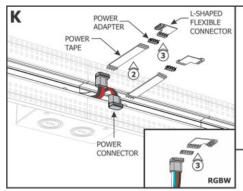
**NOTE:** Omit step 2 for RGBW Configurations. Blank Soft Strip Power Tape is not used.
