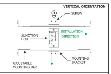
**3:** Mount each adjustable mounting bar to one side of the junction box and secure them with the mounting brackets and two Phillips screws provided.
