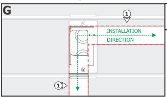
1: Mark and cut out the area where the installation will be located using the junction box opening as a guide (MIN 1.05").
