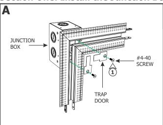
**1**: Remove the #4-40 screws from the junction box to remove the trap door from the assembly using a 1/16" Allen wrench.
