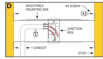
**NOTE:** The adjustable mounting bars mount to studs that are spaced 15" to 24" apart. If the span needs to be shorter than 15", then break the bar arms from dedicated lines.
