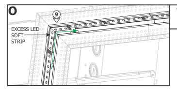
**9:** Trim excess LED Soft Strip ONLY at dashed cutting lines. Overlap excess LED Soft Strip at power connection to avoid dark spots in installation.
