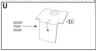
**1**: Use pliers to bend the section of the short trap door cover ~90° to allow for access to power connections.
