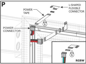
1: Refer to steps 1 through 4 in Section Three to uncoil the LED Soft Strip and connect each power connector to the Blank Power Tape (not used with RGBW), Power Adapter and L-Shaped Flexible Connector.
