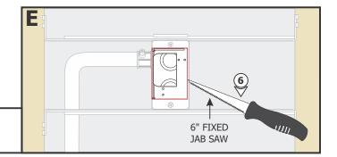
**6:** Cut a section of drywall using a 6" fixed jab saw or other appropriate tool to expose the mounting plate area. Install the drywall.
