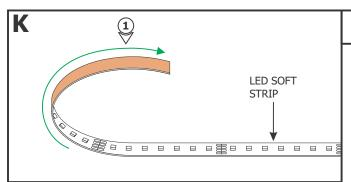
**1:** Gently uncoil the LED Soft Strip before applying to the channel otherwise the strip may lift off of the surface.
