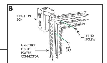
2: Remove the #4-40 screws to remove the L-Picture Frame Power Connector from the junction box using a 1/16" Allen wrench.
