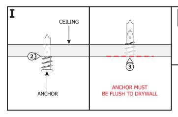
**NOTE:** Steps 2 and 3 are for drywall mounting. Omit these steps if mounting to a wood surface directly.
