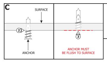
**NOTE:** Steps 2 and 3 are for drywall mounting. Omit these steps if mounting to a wood surface directly.
