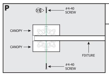
**15:** For 4" Square Split Canopy installations, place each canopy piece against the fixture and align the canopy holes with the crossbar holes. Secure the canopy pieces in place with the two #4-40 screws and 1/16" Allen wrench provided.
