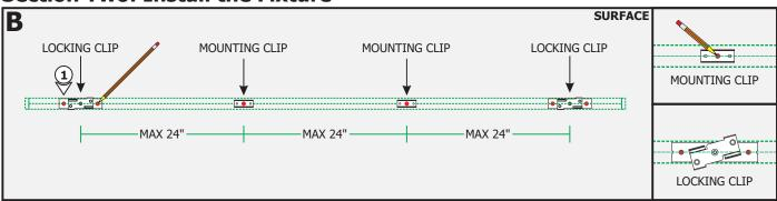
1: Lay the channel to the desired location & make all necessary markings on the ceiling which will consist of the sides and center of the channel, mounting clips and locking clips. Clips must be installed maximum 24" from each other.
