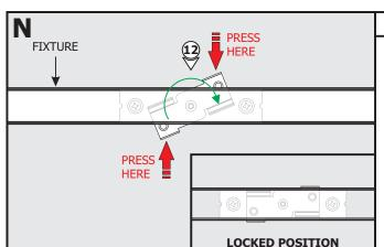
**12:** Twist each locking clip to lock the fixture in place.
