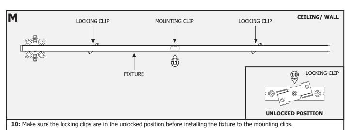
11: Carefully <u>SNAP</u> the channel onto the mounting clips. Make sure not to nick the wires.
