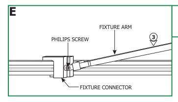
**3:** Rotate the fixture arms to the desired position. If necessary tighten the Phillips screws on the fixture connector to hold the fixture in place.
