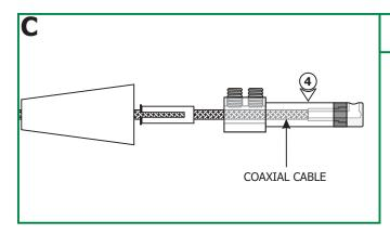
**4:** Feed the coaxial cable into the coaxial fixture connector. The coaxial cable will come to a stop point.
