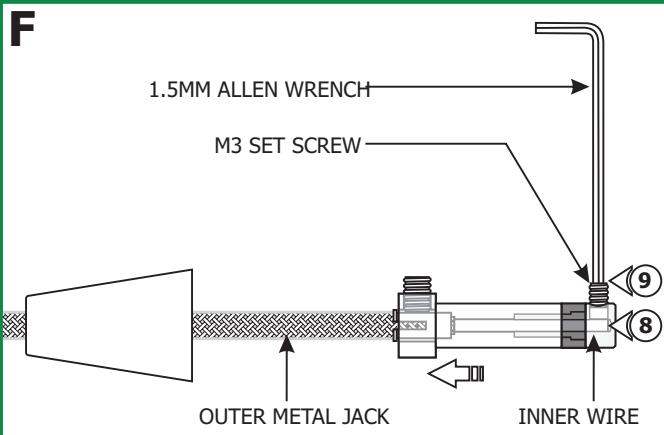
**8:** Keep feeding the coaxial cable in until the inner wire is visible in the screw hole of the fixture connector tip.
