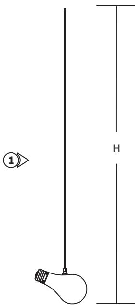
**1:** Cut the coaxial cable to the desired height (H) with a sharp cutter. The overall fixture height is measured from the bottom of the glass shade to the end of the coaxial cable.
