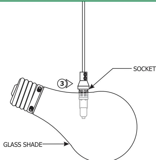
**3:** Push the socket assembly back into the glass shade hole to secure in place.
