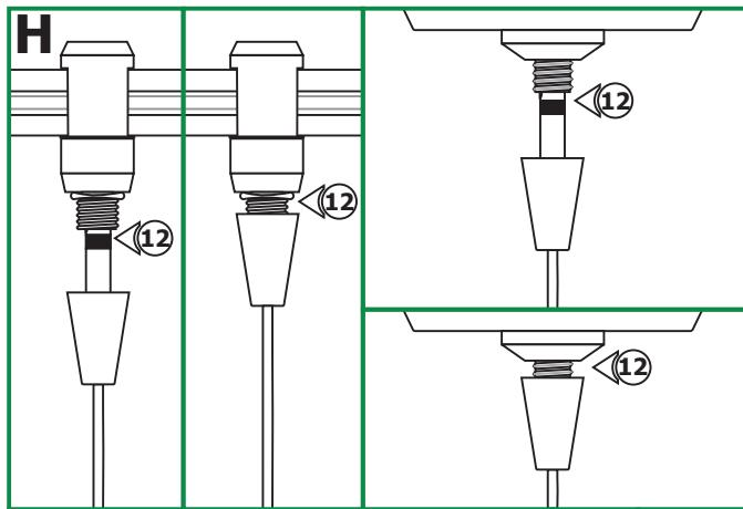
**12:** Use fingers to tighten the Fast Jack fixture connector into the Fast Jack system connector (Monorail, Monorail 2 Circuit, or canopy connector - Refer to the instructions provided with the system connector or canopy).
