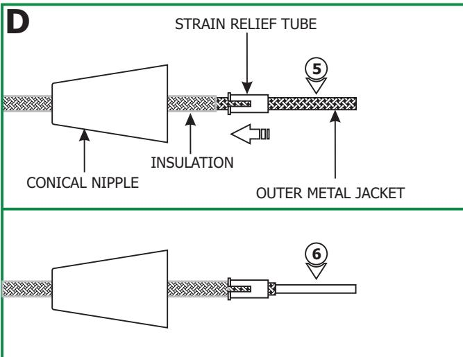
**5:** Feed the coaxial cable through the conical nipple and flared side of the strain relief tube. Slide the conical nipple down the coaxial cable. Slide the strain relief tube against the insulation.
