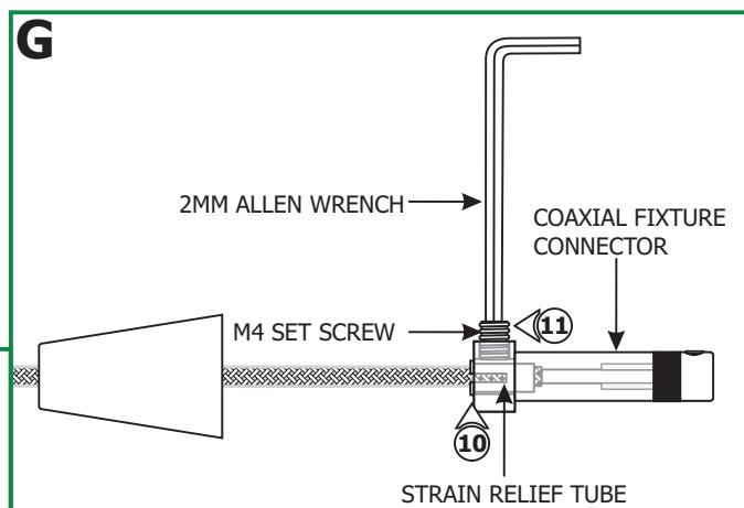
**10:** Make sure the strain relief tube is completely into the coaxial fixture connector and the slot on the strain relief tube is not inline with the M4 set screw.
