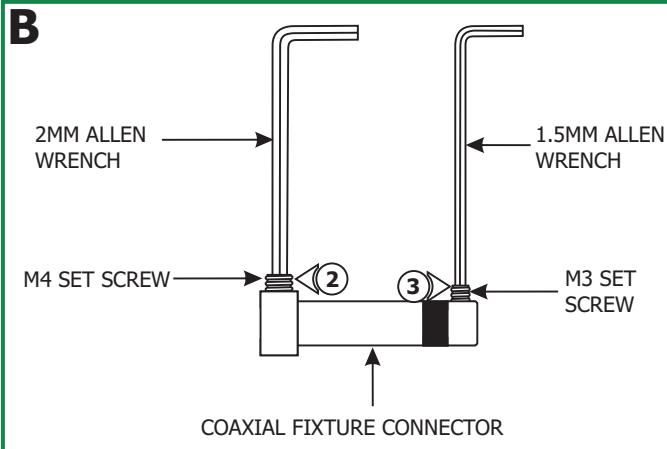
**2:** Loosen the M4 set screw on base of the coaxial fixture connector with the 2mm Allen wrench provided. **Do not remove this set screw.**
