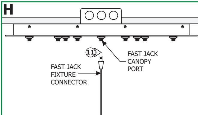
**CAUTION: Risk of Fire:** The total load of the Fast Jack canopy ports should not exceed the remote transformer rated capacity..
