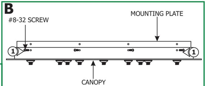
**1:** Remove the sixteen #8-32 screws around the canopy to remove the mounting plate.
