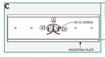
**NOTE:** It is recommended that a person to hold the mounting plate while the electrician installs it.
