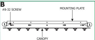
**1:** Remove the fourteen #8-32 screws around the canopy to remove the mounting plate.
