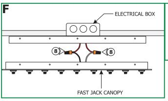
**7:** Make sure that the mounting plate is grounded in accordance with local electrical codes.
