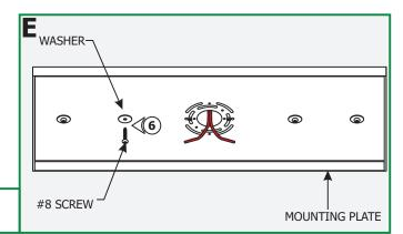
**6:** Secure the mounting plate to the anchors with the provided #8 screws and washers.
