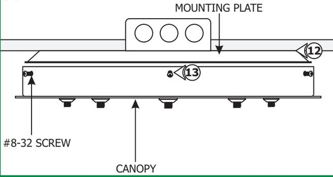
**12:** Place all wires and wire nut connections inside the canopy.
