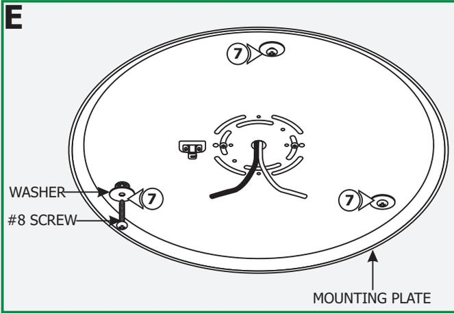
**7:** Secure the mounting plate to the anchors with the provided #8 screws and washers.
