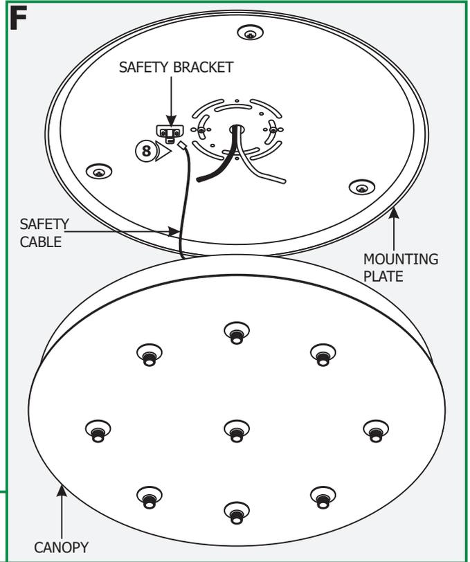
**9:** Make sure that the mounting plate is grounded in accordance with local electrical codes.
