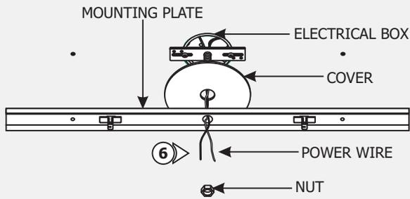
**7:** Slide the cover and mounting plate center hole onto the crossbar threaded nipple and secure it with the nut provided.
