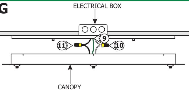
**9:** Make sure the mounting plate is grounded in accordance with local electrical codes.
