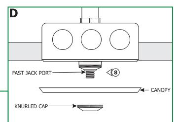
8: Place the canopy center hole onto the Fast Jack port against the electrical box and secure it in place by tightening the knurled cap to the Fast Jack port. Make sure the knurled cap is not cross threaded.
