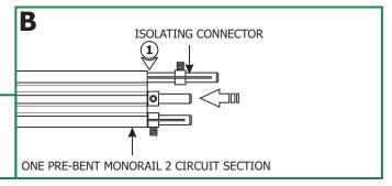
1: Push the straight isolating connectors completely into one pre-bent Monorail 2 Circuit section end. Make sure this pre-bent Monorail 2 Circuit section is secured with the standoffs (Refer to the instructions provided with the standoffs).
