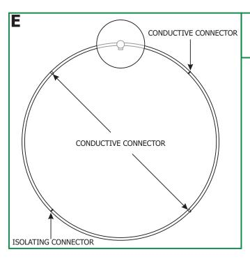
**1: For the Single Power Feed Connection-** Use one set of isolating connectors and the appropriate sets of conductive connectors provided to connect the pre-bent Monorail sections together as a circle.
