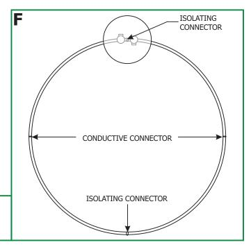
**2: For the Dual Power Feed Connection-** Use two sets of isolating connectors and the appropriate sets of conductive connectors provided to connect the pre-bent Monorail sections together as a circle.
