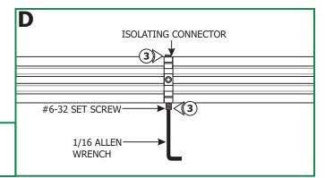
3: Tighten the #6-32 set screw on each of the isolating connectors firmly with the 1/16 Allen wrench. **Do not over tighten the set screws as this may strip the threads.**
