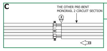
**2:** Push the other pre-bent Monorail 2 Circuit section entirely onto the isolating connectors and simultaneously connect the pre-bent Monorail 2 Circuit to the standoffs.
