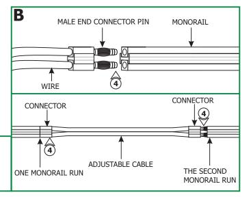
**4:** Push one male end connector pins completely into one Monorail end run, and push the second connector pins of the other side completely into the other Monorail run. Make sure that the Monorail runs are supported by the standoffs. Refer to the instructions provided with the standoffs.
