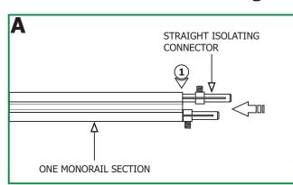
1: Push the straight isolating connectors completely into one Monorail section end. Make sure this Monorail section is secured with the standoffs (Refer to the instructions provided with the standoffs).
