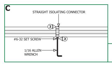
**3:** Tighten the #6-32 set screw on each of the isolating connectors firmly with the 1/16 Allen wrench. **Do not over tighten the set screws as this may strip the threads.**
