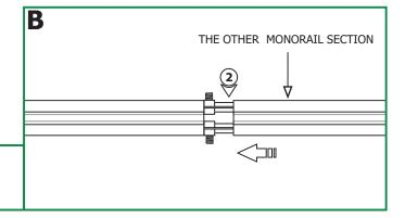
**2:** Push the other Monorail section entirely onto the straight isolating connectors and simultaneously connect the Monorail to the standoffs.
