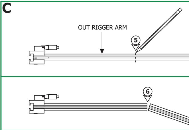
**5:** From the end of the out rigger arm, mark the point where the out rigger arm needs to be shortened. **(Optional)**
