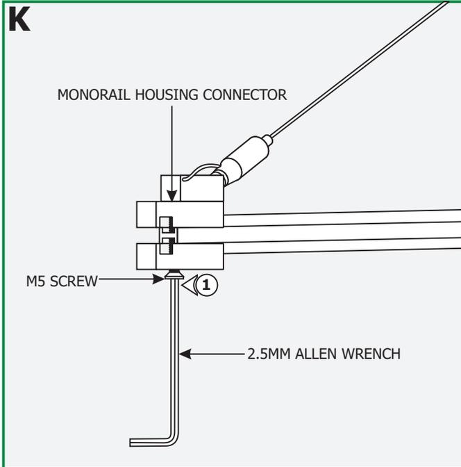
**1:** Slightly loosen the M5 screw on the bottom of Monorail housing connector, (**Do Not Remove**) with the 2.5mm Allen wrench.
