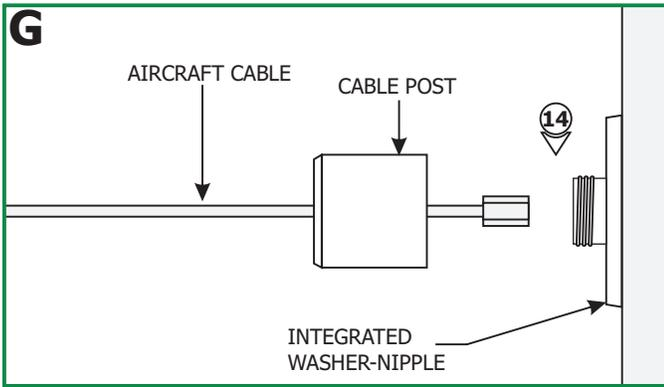
**14:** Feed the aircraft cable through the cable post and screw the cable post completely onto the integrated washer-nipple.
