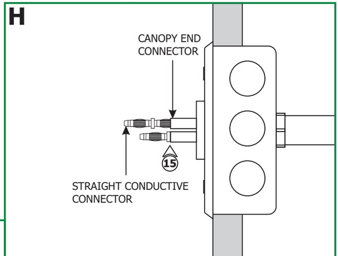
**15:** Push the straight conductive connectors into the canopy end connector.
