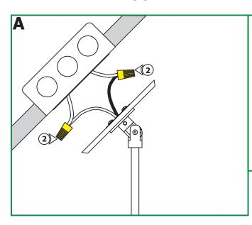
**NOTE:** Use the universal round crossbar (provided) if the electrical box holes are not spaced 2-3/4" apart.
