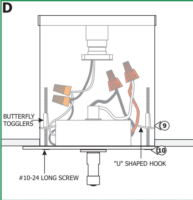
**9:** Align and hang the butterfly toggles onto the "U" shaped hooks on both sides of the down lights.
