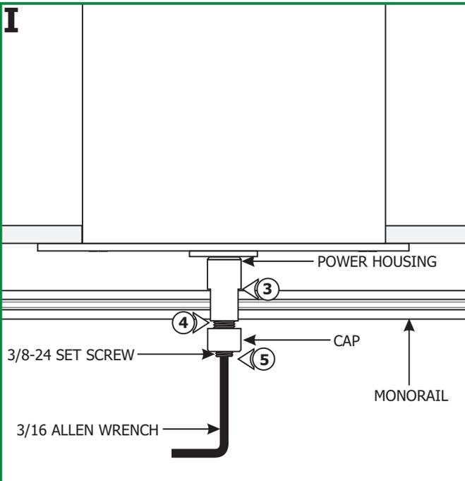
**3:** Place the Monorail into the power housing and support it with the standoffs (refer to the instructions provided with the standoffs).
