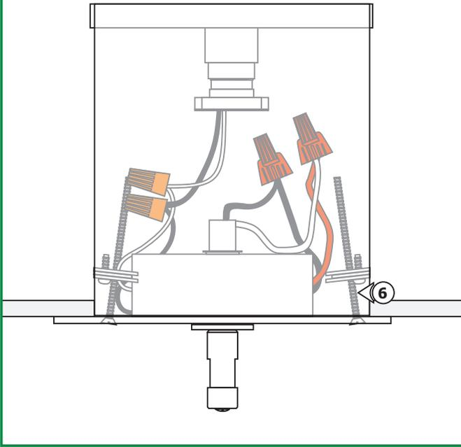
**6:** Screw the #10-24 long screws into the center hole of brackets.
