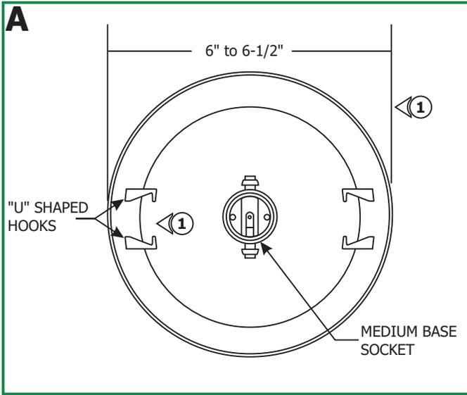
**1:** The Monorail recessed can transformer can be mounted to down lights that:
