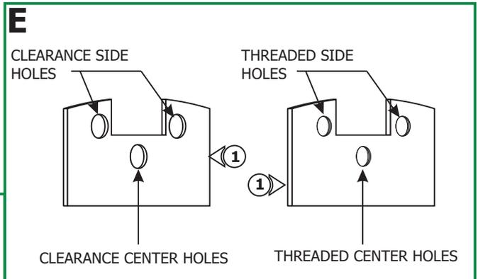
**1:** There are four mounting brackets included in the package, two of them with threaded holes and two others with clearance holes. Each set uses a threaded and a clearance hole brackets.
