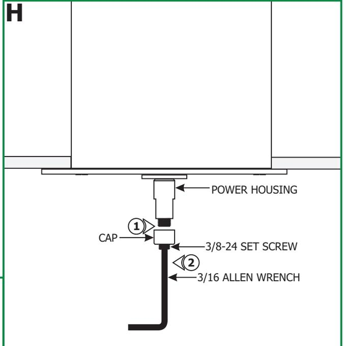
**1:** Unscrew the cap from the power housing.
