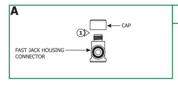
1: Remove the cap from the Fast Jack housing connector.
