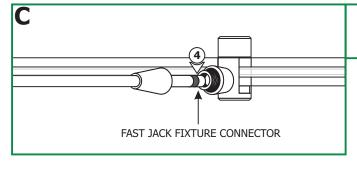
**4:** Push the Fast Jack fixture connector into the Fast Jack housing connector.
