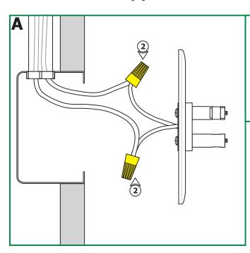
**NOTE:** The low voltage wires should be present in the electrical box. Refer to the instructions provided with the remote transformer to install the transformer and the low voltage wires before proceeding with the steps below.
