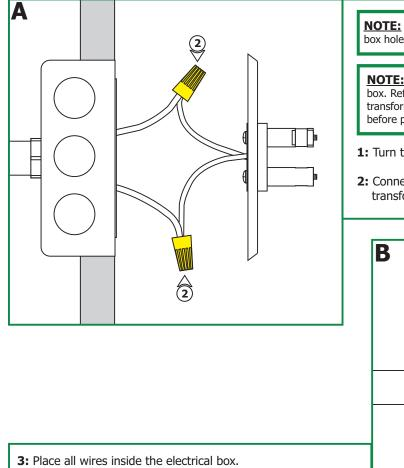
**NOTE:** Use the universal round crossbar (provided) if the electrical box holes are not spaced 2-3/4" apart.
