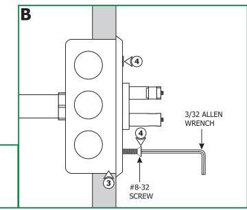
4: Secure the power feed canopy to the electrical box by tightening the two provided #8-32 screws with the 3/32 Allen wrench.
