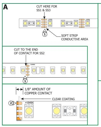
**NOTE:** The goof connectors are used to connect two soft strips together when the ends are cut by accident. Please note that when joining two cut section of the soft strips together, the total length of the soft strip should not exceed the maximum allowance as is indicated in soft strip spec sheet or the installation instructions.
