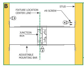
**NOTE:** The adjustable mounting bars mount to studs that are spaced 13" to 24" apart.
