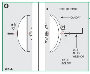
**10 (OPTIONAL):** For 4" Round Canopy installations, place each canopy piece against the crossbar and secure it to the electrical box holes with the provided #4-40 screws using the 1/16 Allen wrench.
