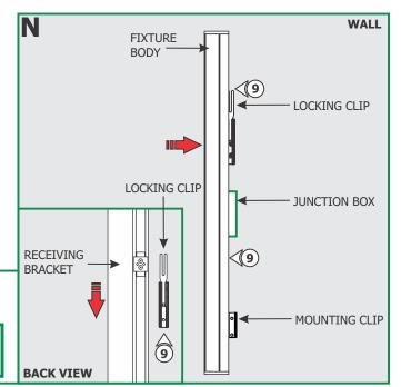
**9:** Carefully snap fixture body onto the locking & mounting clip(s) then slide into receiving bracket to lock in place. Make sure not to nick the wires.
