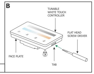
**3:** Pry the face plate of the Tunable White Touch Controller using a flat head screw driver.
